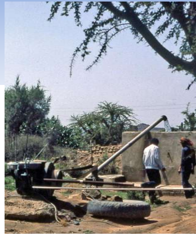
Diesel-powered pumped irrigation well
