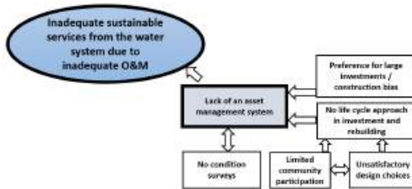
Figure 18 One of the root causes for the BNR cycle: The lack of an asset management system
