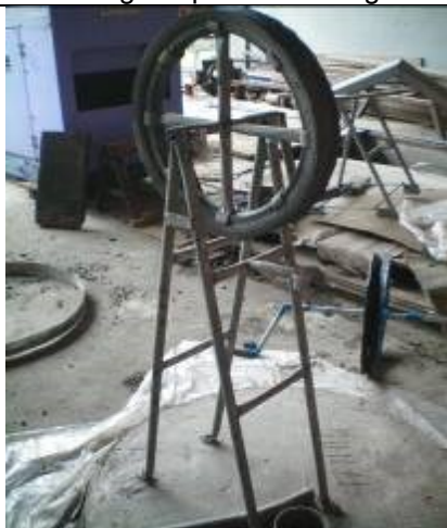
Mounting of Rope pump Model 2. A frame, economy model. Instead of welding angle iron and rebar, legs are bend and have a hole so less material and less welding
