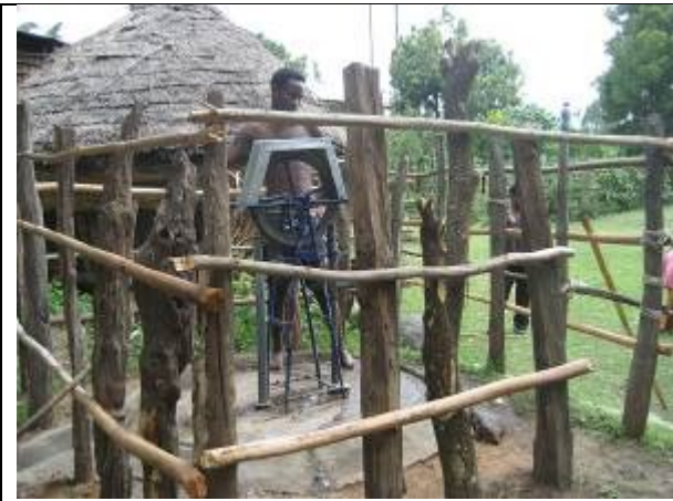
Rope pump protected from Cows
