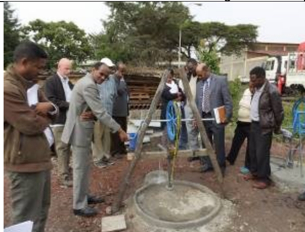
Rope pump model 2. Cost 100-150 US$. The model 1 is similar but has ball bearings
