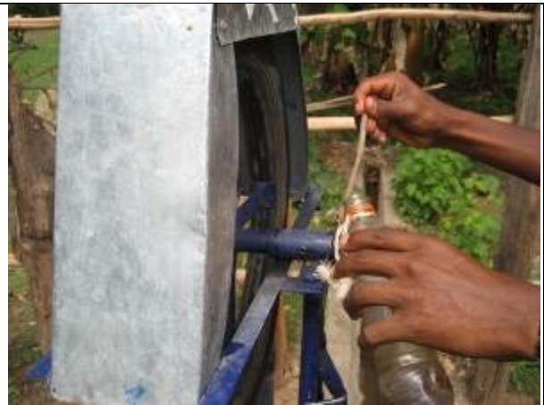
Lubrication of bushings. To make it easier oil hole should be on top
