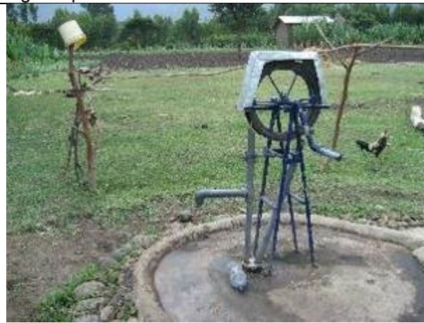
Model 1 Bushings, Bend legs. Pump pipe and return pipe via the 4 inch pipe. Improved model
