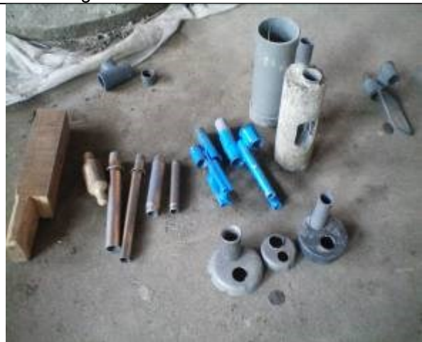
Jigs and tools produced during mission Incl. socket and trumpet tools, end caps, cement guide block.
