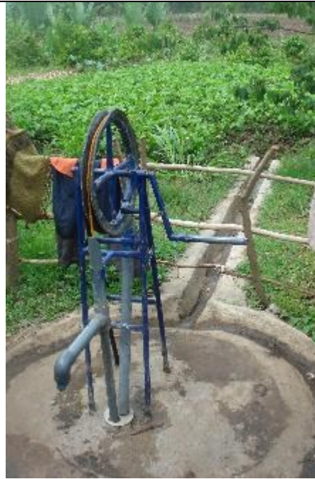
Several pumps were used for productive use. Here the pumps is used for irrigation of a garden of 300 m2
