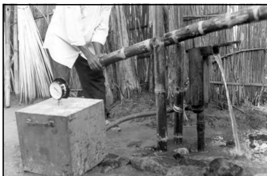
Figure 8 Vacuum gauge reading on a treadle pump to determine well filter resistance
