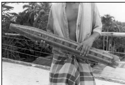
Figure 4 A bamboo filter with mosquito net wrapping
