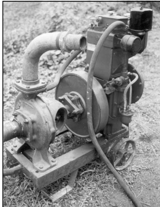
Figure 1 Typical 5 hp/1500 RPM diesel pump, before modification
