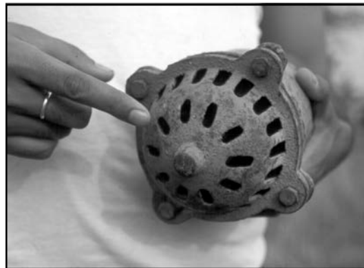
Figure 6 The high-friction foot valve as used on dug wells or pumping from surface water
