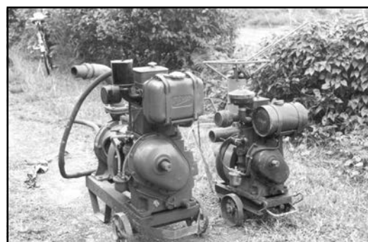
Figure 12 The improved 2.5 hp pump set next to a common 5 hp pump set
