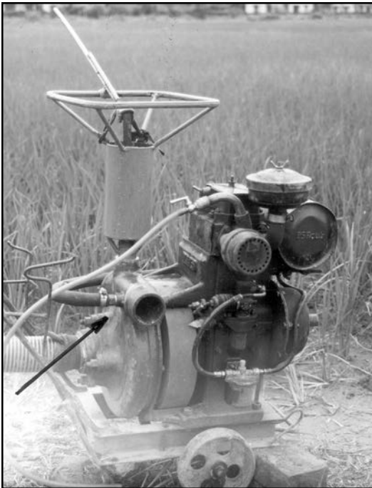
Figure 11 Half-pipe for creating cooling water flow pressure
