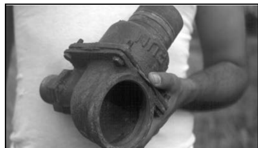
Figure 4 The high-friction check valve as used on shallow tube wells
