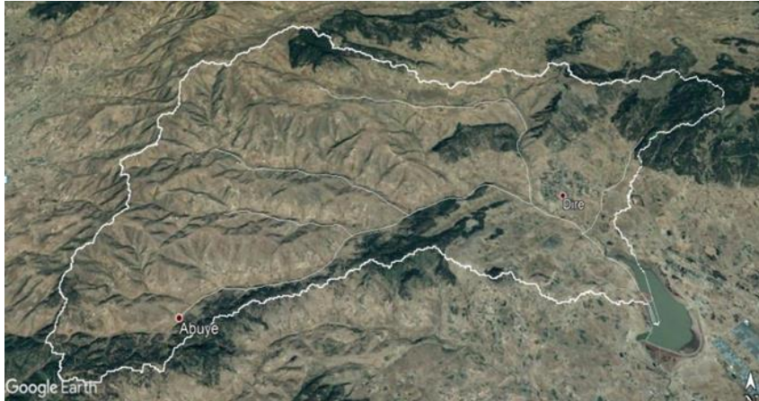
Figure 5.1 Delineation of Dire Dam Water Catchment
