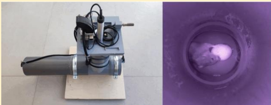
Figure 5: SPYCE device developed in MED4PEST (left); image of rodent activity captured by SPYCE (right). (Photo credit: HMU)
